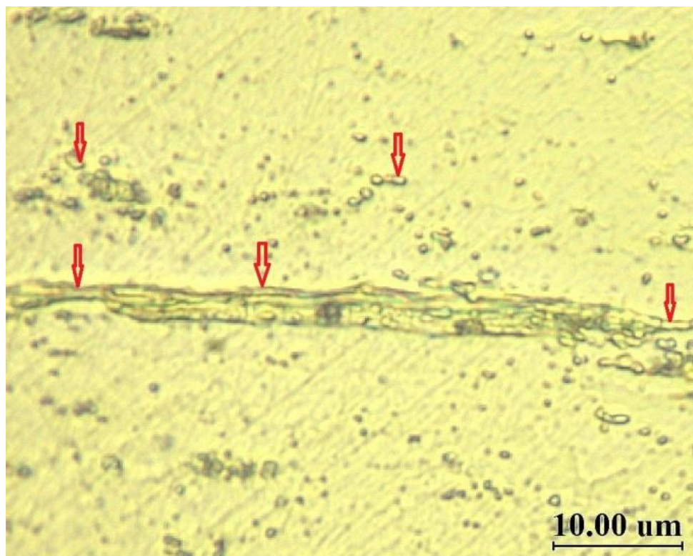
Fig. 3. Microstructure of aluminum composites reinforced with GNPs extruded at 400 °C and annealed at 610 \pm 10 °C during 3h. Black arrows indicate GNPs, red arrows indicate carbides
