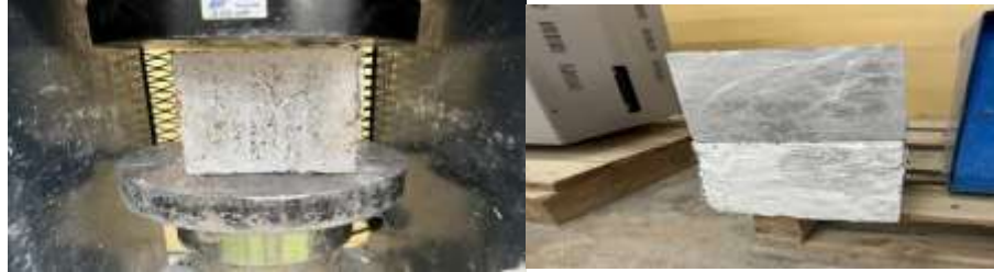
Figure 4.3: Compression testing of SIFCON specimens.
