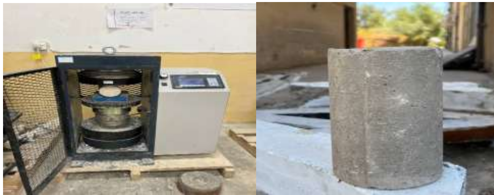
Figure 4.4: Tensile testing setup for cylindrical concrete samples.
