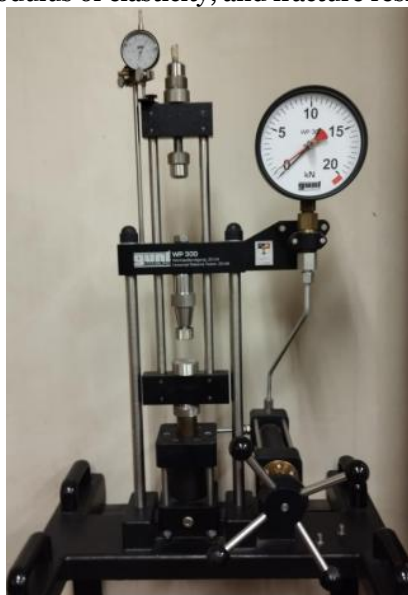
Figure 2: Gunt Hamburg WP300 Universal Testing Machine
