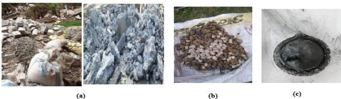
Fig 2: Photos (a) C&D waste (b) Crushed C&D Waste (c) Graphene used
