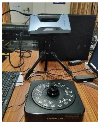
Figure 1 :3D Scan setup of structure light based scanner.
