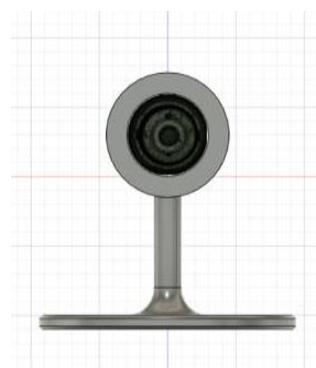
Figure 4 : Assembled model of security camera (virtual camera and 3D designed support stand model).
