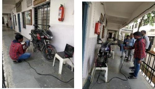
Figure 5 : 3D scanning operation by using the structured light scanner and photogrammetry process.
